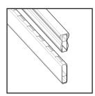
Measure from inside edge between Posts subtracting 1/4" (1/2" for \*non-standard stair angle) from total length, and if necessary cut Rail/ Rail Insert to proper length by cutting an equal amount from each end. Do not cut through Baluster holes
