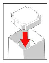
Insert Balusters into the holes in the Bottom Rail. Push firmly to set.
