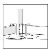
Measure between Posts subtracting 1/4" from total length, and if necessary cut Rails and Rail Insert to proper length by cutting an equal amount from each end. Do not cut through Baluster holes.
