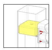
Place Top Rail with Rail Insert 36" or 42" (measured from the deck surface to the top face of the Rail), and onto Balusters. Fasten to center of Post with provided screws ensuring at least one screw on either side of the rail penetrates the poly block. Secure Bracket to railing then slide Screw Covers into place.
