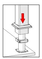
Space Posts according to deck configuration and Top Rail length.
