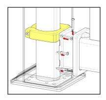
**Tip:** Cut a block to 2" and set Bottom Rail on it for support during installation
